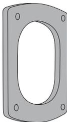
**Note:** When using a 435VFSM or 435VFDM mounting flange, the black rubber gasket supplied with the mounting flanges must be inserted into the back recess of the 415VF or 435VFS15 product as shown. The foam gasket supplied with 415VF or 435VFS15 product should be mounted on wall surface regardless if mounting flange is used.
